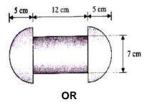
8. The cross-section of a plain concrete culvert as shown in fig. Determine the moment of inertia about the horizontal centroidal axes.
