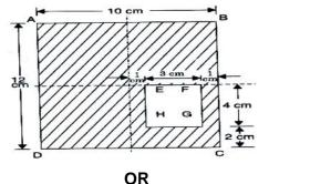
8. Determine the centroid of the composite area as shown in figure. All dimensions are in mm.
