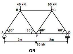
4. A truss of 8 m span and 4 m height is loaded as shown in Fig. Find the magnitude and nature of the forces in all the members.
