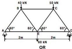
4. A simply supported beam is loaded as shown in figure. Find the reactions.
