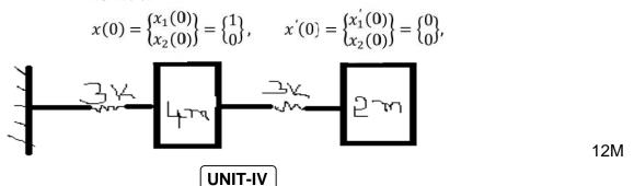
7. Find the lowest natural frequency of the following system using stodola method
