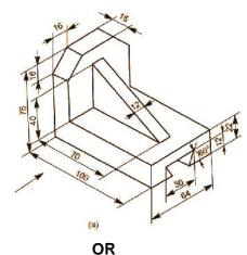
10. The Figure shows an object. Draw its (i) Front view (ii) Top view (iii) Side view. Assume all the dimensions are in 'mm '.
