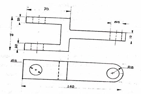
8. Consider the picture shown in figure below and draw the front view, top view and side views in first angle projection.
