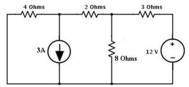
2. a) Using mesh analysis find current through 4 resistor.
