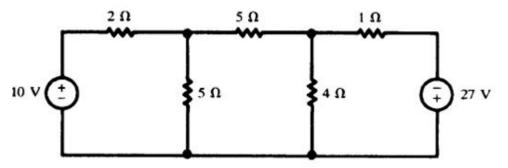
b) Determine the current in the 2 resistor for the circuit shown below, by using nodal analysis.
