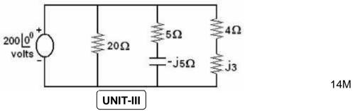
5. a) Derive an expression for the resonant frequency for a parallel circuit shown below
