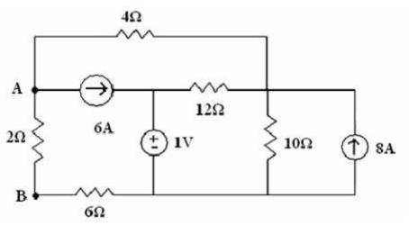
b) Find the current i in the circuit shown in fig, given below using superposition theorem
