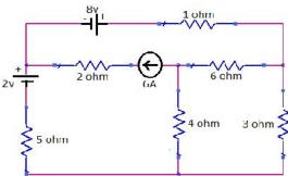
b) Determine the node voltages and current through each resistor for the circuit shown in fig
