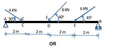
4. Draw the shear force and bending diagrams for the beam shown loaded in fig. Clearly mark the position of the maximum bending moment and determine its value.
