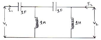
b) Determine the Z parameters for the network shown.
