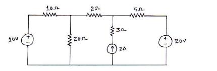
b) Determine the value of resistance R in the network shown for maximum power transfer to it and the maximum power.
