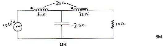
10. a) Draw the graph of the network shown and select a suitable tree and obtain the cutset matrix. Also write KCL equations from the matrix.
