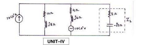
7. a) In the arrangement of figure shown below, find the ABCD parameters of N<sub>0</sub>.
