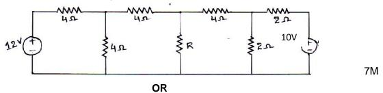
6. a) Calculate the current flowing through Z<sub>L</sub> by applying Millman's theorem in the network.
