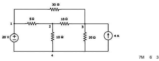
b) Define i) link ii) Twig iii) tree iv) co-tree with a suitable diagram
