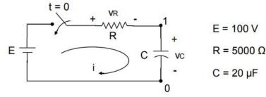
b) Derive the current expression in RC series circuit excites by constant DC voltage Source after closing the switch at t=0
