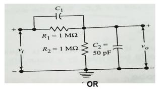
The square wave shown in figure is fed to an RC coupling network. What are 2. a) the output voltage wave forms if a) RC =10T b) RC = T/10
