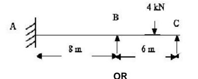
7. Analyze the continuous beam shown in **figure** by moment distribution method. Draw the SF and BM diagrams.
