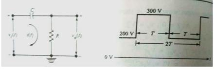
b) A 1kHz symmetrical square wave of ± 10V is applied to an RC circuit having 1ms time constant. Calculate and plot the output for the RC configurations as a) high-pass circuit and b) Low-pass circuit
