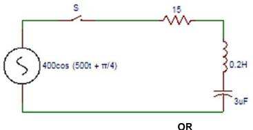
6. a) The circuit shown in the figure consists of resistance, capacitance and inductance in series with a 100V source when the switch is closed at t = 0. Find the equation obtained from the circuit in terms of current.
