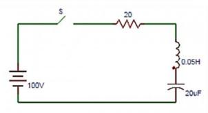
b) In the circuit shown below, if current is defined as the response signal of the circuit, then determine the transfer function.
