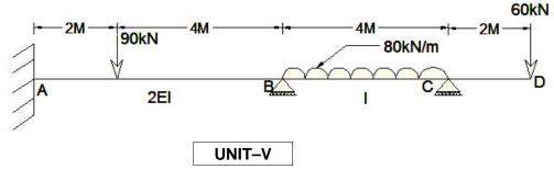
9. Analyze the continuous beam shown in fig. below by plastic Analysis. All the loads are service loads, use partial safety factor of 1.5
