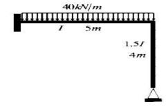
6. Analyse the beam shown in fig. below by using Kani's method. EI=Constant
