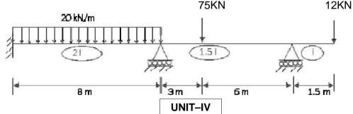
7. a) Analyze the beam shown in figure by flexibility matrix method
