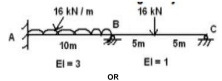
8. Analyze the continuous beam shown in figure using stiffness matrix method and draw the bending moment and shear force diagrams
