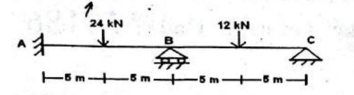
b) Analyse the continuous beam ABC shown in Fig below by flexibility matrix method and draw the bending moment diagram.  $R_B$  and  $R_C$  are redundant
