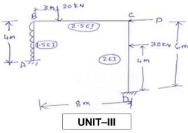
5. Analyze the continuous beam shown in fig. below by Kani's method. El=constant.
