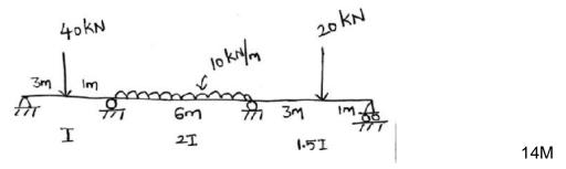
6. Determine the reactions at the supports A, B and C, then draw the shear and bending moment diagrams. Assume EI is constant.
