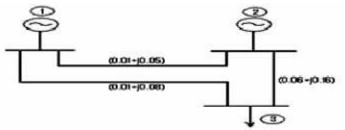
Slack bus-1: V=1.05+j0.0 P-V bus-2: V<sub>2</sub> =1.03 pu : P<sub>2</sub> =0.5 pu; 0.1< Q<sub>2</sub>>0.3 Load bus-3: P<sub>3</sub>=0.6pu ; Q<sub>3</sub>=0.25pu
