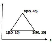
For the axisymmetric element shown in figure, determine the element stresses.
