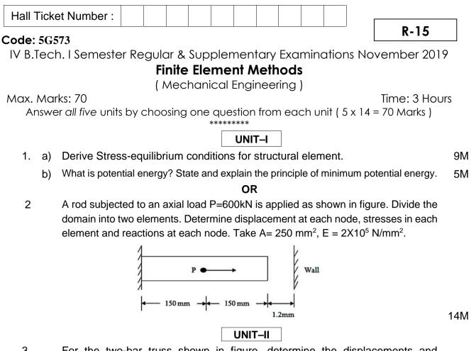
3. For the two-bar truss shown in figure, determine the displacements and stresses. A<sub>1</sub>=500mm<sup>2</sup>, A<sub>2</sub>=1200mm<sup>2</sup>, E=2x10<sup>5</sup> N/mm<sup>2</sup>.
