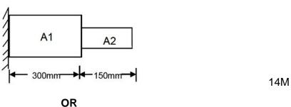
10. Evaluate the lowest Eigen value and the corresponding Eigen modes for the beam shown in figure. E=200 GPa and <sup>...</sup> =7840kg/m3, I=2000 mm4, A=240 mm2, L=300mm.
