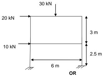
10 Find out the plastic moment of given frame by combining mechanics method.
