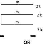
8. Determine the natural frequencies and mode shapes shown in Fig by Holzer's method.
