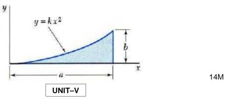
9. Determine the moments of inertia and the radius of gyration of the shaded area with respect to the x and y axes.
