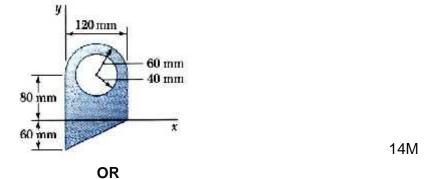
8. Determine coordinates of the centre of mass of lamina given below:
