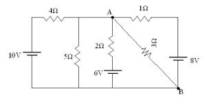
8 Find the voltage across  $4\Omega$  resistor in the circuit shown using Superposition theorem and also verify it using mesh analysis.
