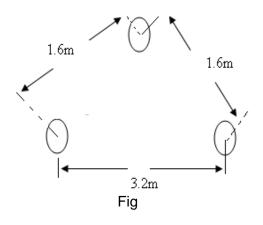
2 An overhead 3- $\Phi$  short transmission line delivers 4000 kW at 11 kV at 0.8 pf lagging. The resistance and reactance of earth conductor are 1.5 $\Omega$  and 4 $\Omega$  per phase respectively. Determine:
