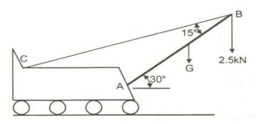
Determine the axial forces in the members of plane frame as shown in the below figure.
