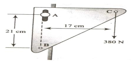
2 Determine the induced forces in each members of the frame as loaded and supported as shown in the below figure.
